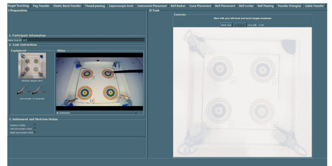
Figure 3: Task GUI in MEVIS Lab -- For the later study, we coupled a MIDI interface (sonifications) and the simulator interface (camera, instruments).
